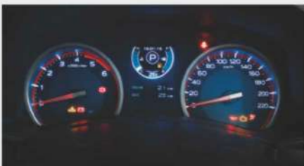
3D Electro-luminescent Instrument Cluster with Multi-information Display
